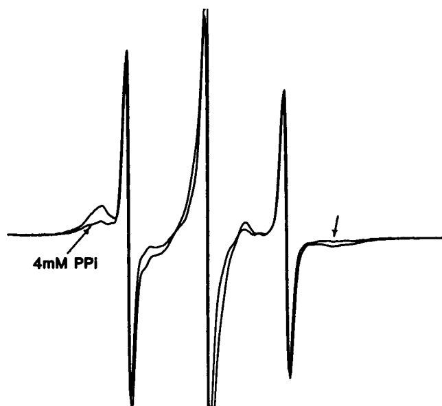
FIGURE 5 EPR spectra of unlabeled fibers in the presence of 50 \mu\text{M} SL-ADP rigor buffer, 20^\circ\text{C} , with 0 and 4 mM MgPP i . The three sharp peaks come from analogue that is not bound to protein. Broad peaks at low and high field are from SL-ADP bound to the nucleotide site. Addition of MgPP i , which competes for the nucleotide site on myosin, decreases the intensity of the broad peaks due to bound SL-ADP by \sim 50\% , allowing one to calculate the affinity of MgPP i for the actomyosin complex.
